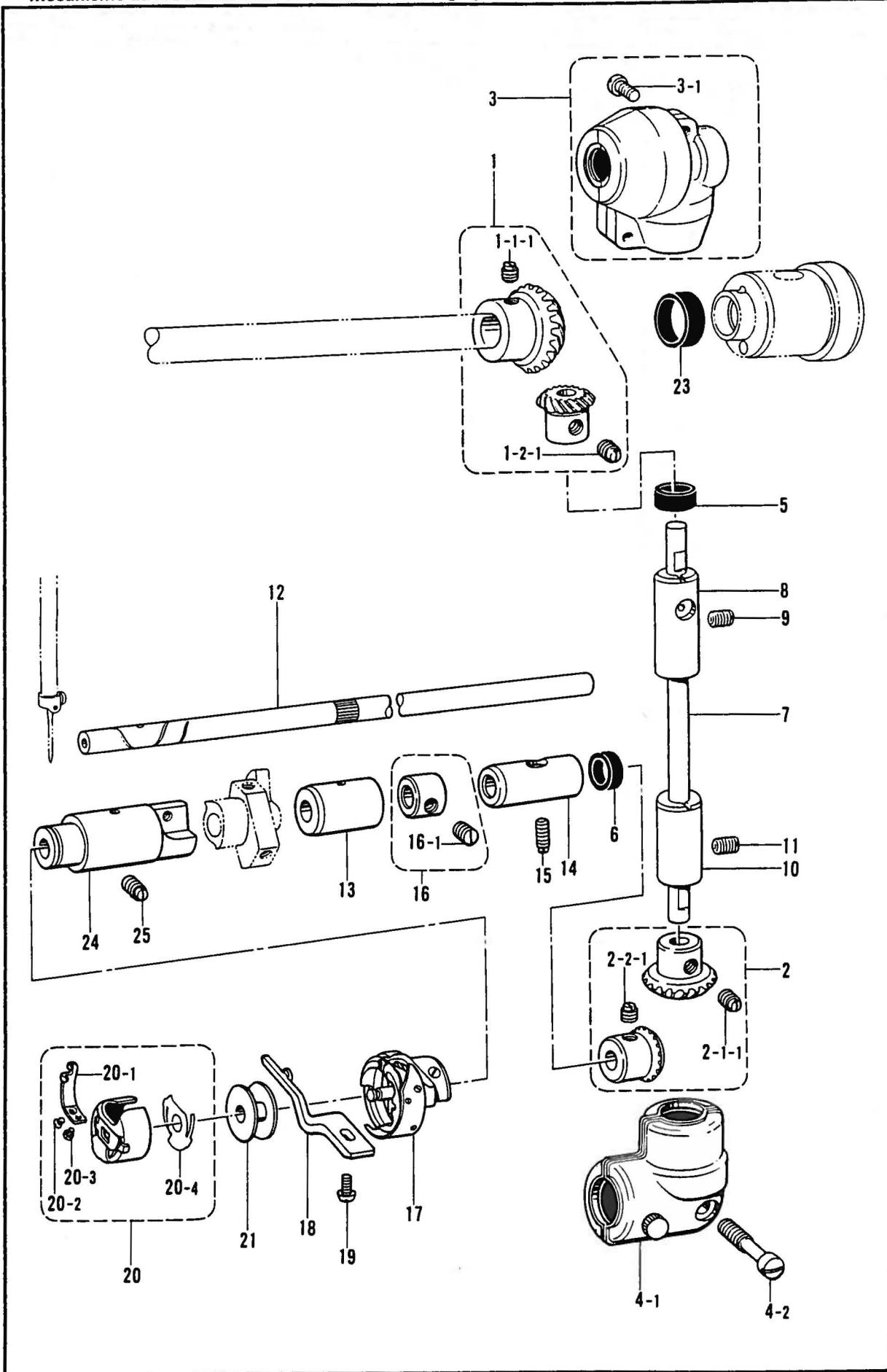
H. カマ関係/Rotary hook mechanism/Greifervorrichtung/
