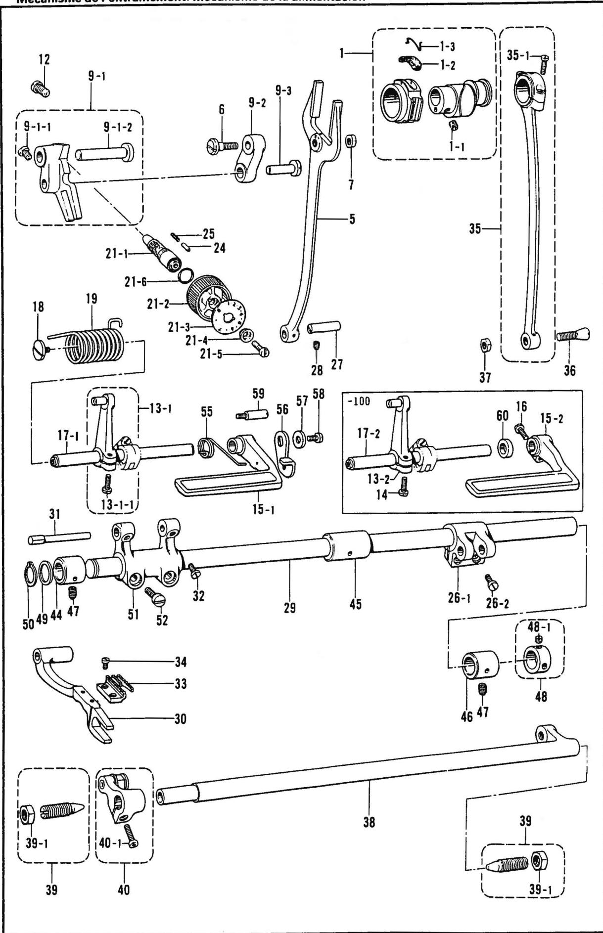
F. 送り関係/Feed mechanism/Transportvorrichtung/
